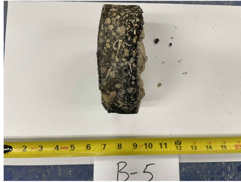
P-5: 1.5 INCHES THICK ASPHALT
