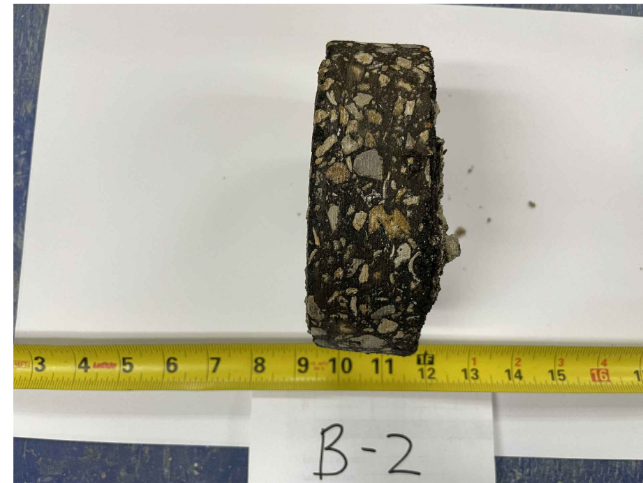
B-2: 1.75 INCHES THICK ASPHALT
