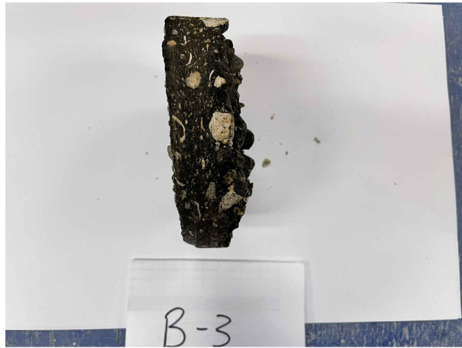
B-3: 1.0 INCHES THICK ASPHALT
