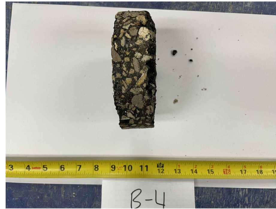
B-4: 1.5 INCHES THICK ASPHALT
